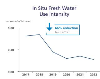
Includes Alberta thermal in situ facilities. In situ fresh water use intensity has decreased from 2021 due to increased use of treated process water and saline water sources in operations.
