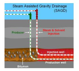
In typical SAGD oil production, water is heated to create steam that mixes with the bitumen and improves its viscosity so it can be pumped to the surface. When solvent is added, the SOR is significantly decreased. At Primrose, in the steam flood area, a solvent injection two-year pilot commenced in Q4 2021. This pilot consists of nine net wells (five producers and four injectors), targeting SOR and GHG intensity reductions of 45% and solvent recoveries of greater than 70%.
