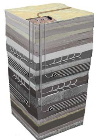
Multi-lateral horizontal and fishbone wells.
